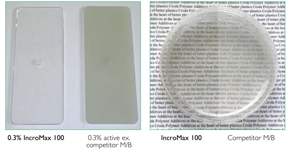
Figure 4: 2mm thick molded PET plaques containing 0.3% IncroMax 100 and 0.3% active ex. competitor masterbatch for colour comparison
